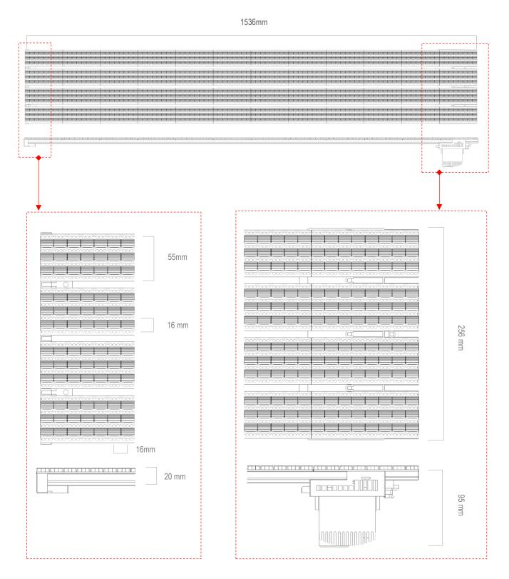
NOTE: 1. The size is a standard size, the length of the unit is customizable and the height is not customizable ;
